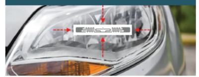
Peel headlight tag from protective plastic backing and apply sticky side to MIDDLE OF HEADLAMP being sure to mount the tag level to the ground.
